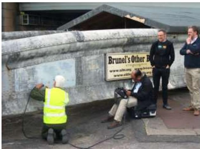
Plate-thickness measurements have been carried out by our volunteer friends from the British Institute of Non-Destructive Testing using Ultra-Sonic test equipment. Subsequent tests using sophisticated Pulsed Eddy Current equipment were carried out courtesy of Baugh & Weedon.
