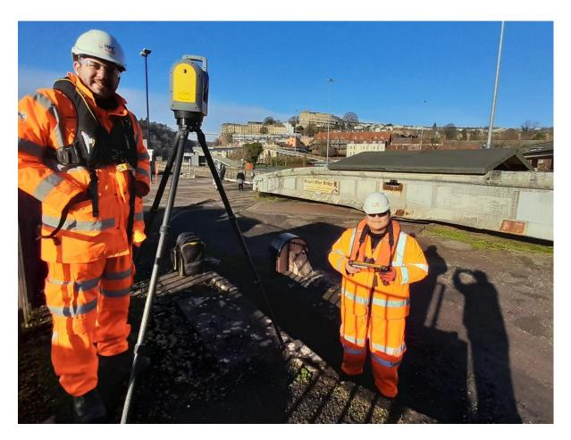
For the technically-minded, a Trimble X7 scanner and software were used, controlled from a portable tablet via a local W-Fi connection. The fully automated equipment simultaneously scanned and photographed, rotating 360° in three dimensions.
