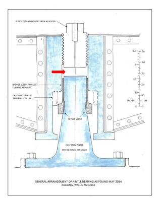
Brunel intended that a large part of the weight of the rotating deck should be carried by a central bronze pad sitting on a pointed casting called a 'pintle'. This literally means 'little pin' although it is, in fact, a heavy casting nearly a metre high.
