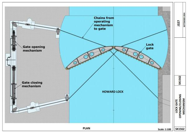
When the lock gates were installed in the 1870's they may have been operated by some form of winch or early hydraulic system. Then around 1903 hydraulic gate opening and closing mechanisms were fitted, as illustrated on our volunteer Bob Watkins's excellent drawing above. Heavy chains passed down into the lock and pulled the lock gate open, whilst another similar system pulled the gate closed. Thus eight sets were installed to operate two pairs of gates, **AND MOST STILL SURVIVE!**
