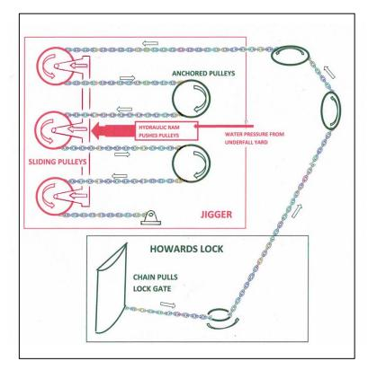
The mechanisms are called 'jiggers'. They comprise giant hydraulic rams were supplied with water compressed to 750 psi (5.1 MPa) via cast iron pipes from Underfall Yard where the contemporary pumps are still working. The water operated a piston ('ram') which pushed three pulleys with chains round them as illustrated left.
