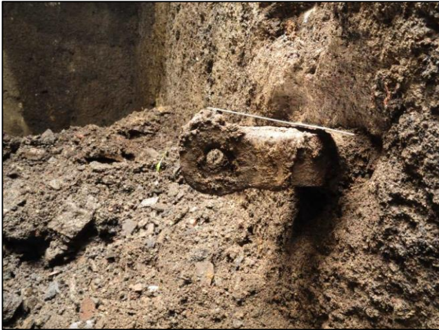
Photo 8 – View of the side of the clip, showing the 1¼" diameter hole that runs through both arms.
