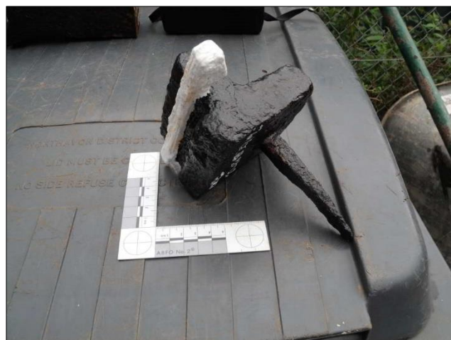
Photo 5 – The latest example of Dramway rail chairs after conservation. The rail fixing spike was still attached and has been painted white. (5 cm x 5 cm scale)
