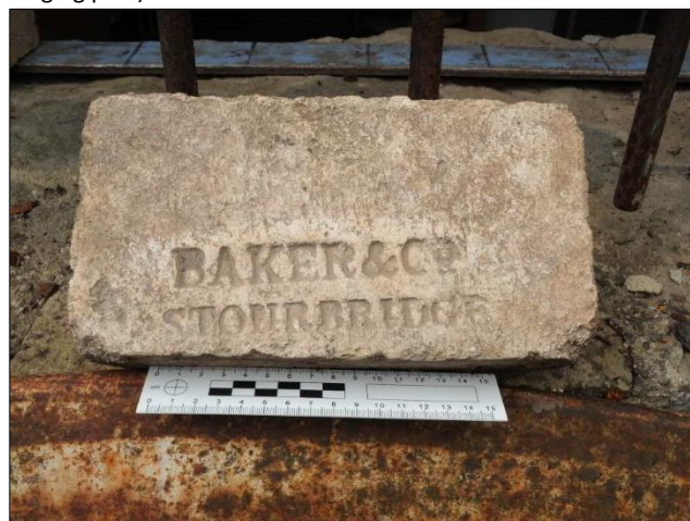
Photo 19 – This firebrick was found when cleaning out the extension of the flue to the north-east of the Egg-ended Boiler settings. We have not found any information on the maker at the time of writing. (15 cm scale)
