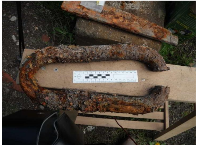
Photo 32 – This artefact, which looks like a link from a standard three-link coupling, was found in the area seen in photo 30. It looks as if it has been deliberately cut open to detach it from the others. (15 cm scale)
