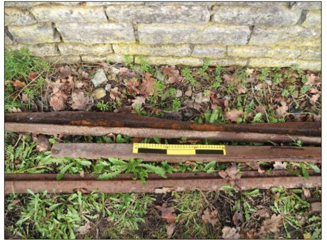
Photo 55 – Two lengths of fish-bellied rail, top and middle, with a length of top hat rail at the bottom. (30 cm scale)
